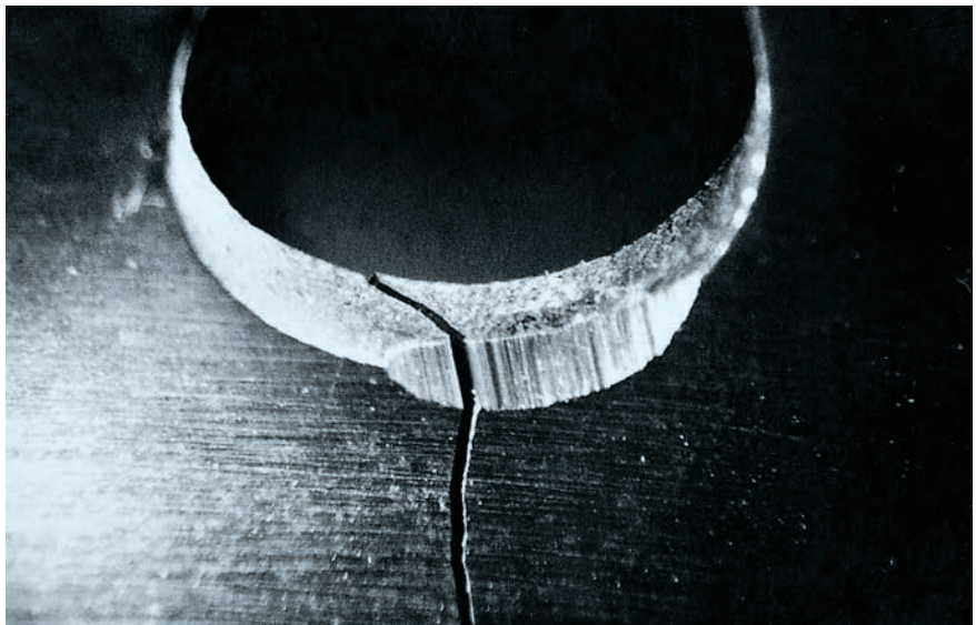
Fracture in the saw body.
