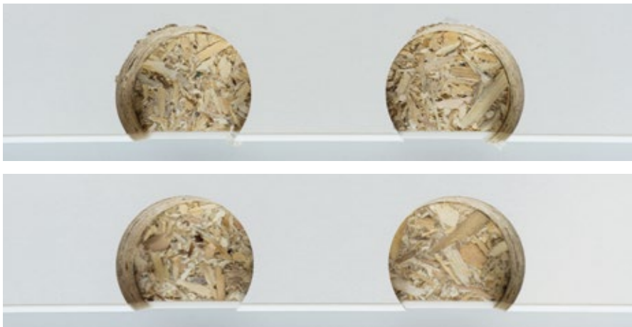
Picture above: Holes for furniture hinges with conventional hinge boring bits.
