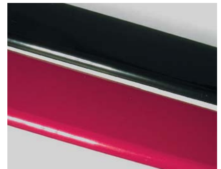
Finish with Leitz Duo-Multi-Profile scraper
