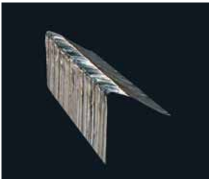
Sharp-edged wear on a coated HS edge
