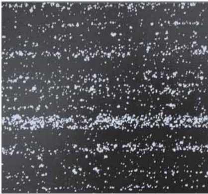
Roco-shaped structure of HS steel made by a molten metallurgical process
