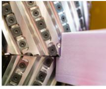
The HeliCut system is perfect for the side processing of insulation panels.
