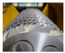
Not only the teeth, but also the gullet area of the circular sawblades are made of solid tungsten carbide and thus effectively prevent washing out of the tool body. This results in excellent durability and a maximum tool life.
