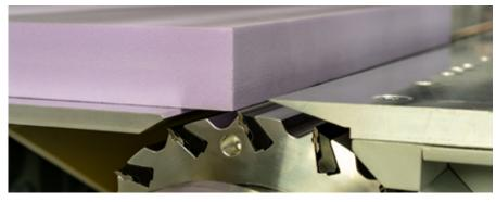
The CentroFix system with its changeable knives is very service-friendly and produces an excellent finish quality in nearly all XPS and EPS foams.
