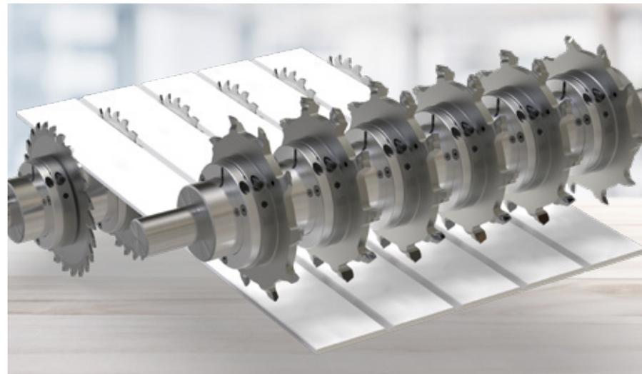
Frequently, the positioning of several tools on a single spindle is implemented by using spacers and the securing is done by a spindle nut. Due to some of the faces not being 100% square or contaminated, the shaft can become distorted. In addition, resetting to other workpiece dimensions can be very time-consuming.
