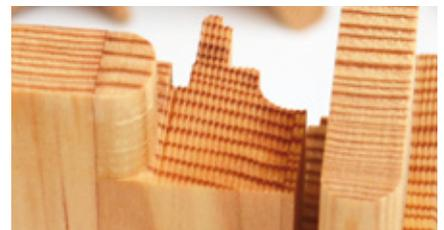
Typical surface with RipTec, without tear-out
