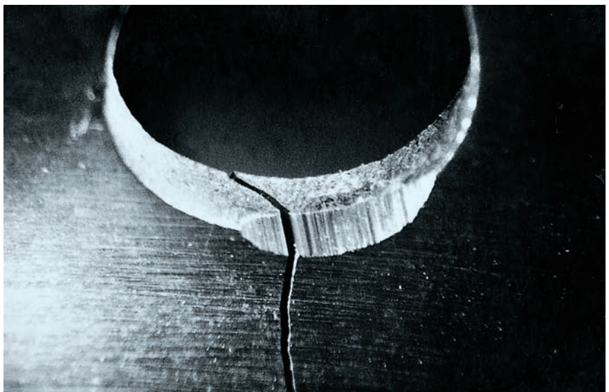
Fracture in the saw body.
