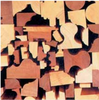
Manufacturing profiled mouldings is important. Profiled mouldings are used, for example, at floor level as skirting boards, around doors as frame profiles, and in cabinetry as decorative mouldings. Such products are usually manufactured on four-sided moulders on through-feed machines and pose specific requirements on the tool system.
