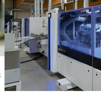
For the edgebanding lines, Leitz has exclusively developed a jointing cutter for laser edges, which even allows the processing of 8 mm panels
