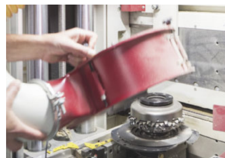
To reposition the cutting edges, the dusthood must be released
