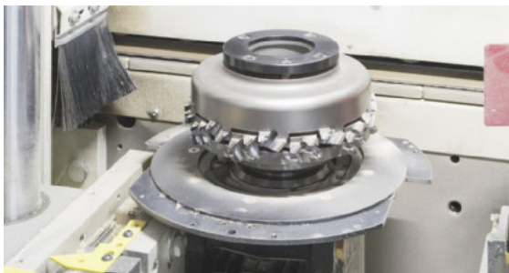
The jointing cutter is exposed and can be easily adjusted from above with the Allen key
