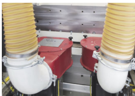
... the second and third jointing cutter in "with feed" direction for 16 or 19 mm front panels
