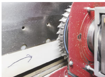
Hoggers remove the bulk of the material and relieve the jointing cutters
