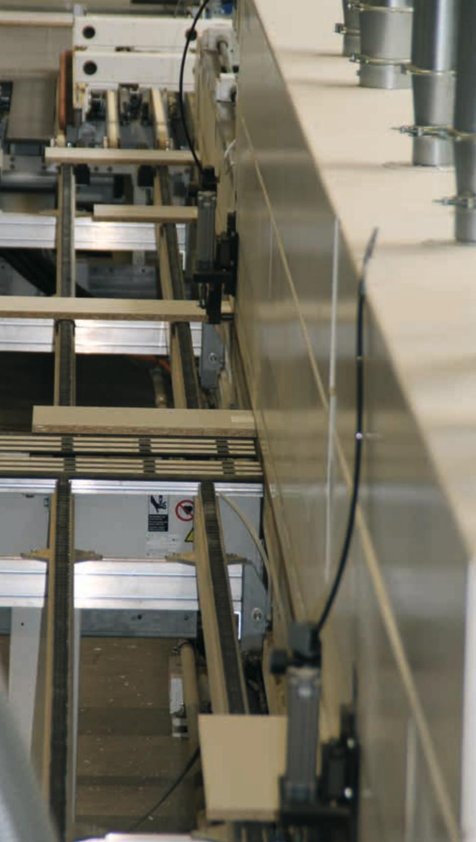
Regardless of size: the system measures the parts' thickness before the format cut, the axes then automatically move to the exact value of the upper edge. Thanks to laser edges, colour changes can be made super quickly.
