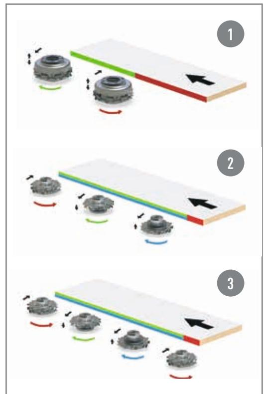
Thus, the Leitz tool system for edge processing during laser jointing at Hunger has changed over the years: It started with a double jointing. Then came machining with three milling cutters. Finally, the step to four tools
