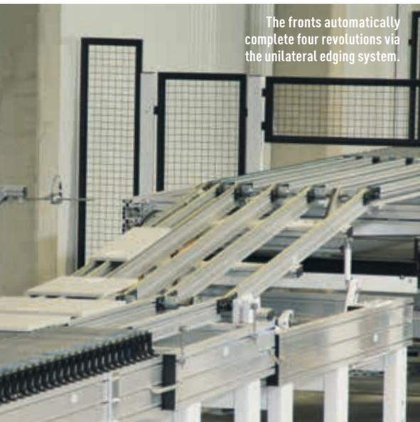
The fronts automatically complete four revolutions via the unilateral edging system.
