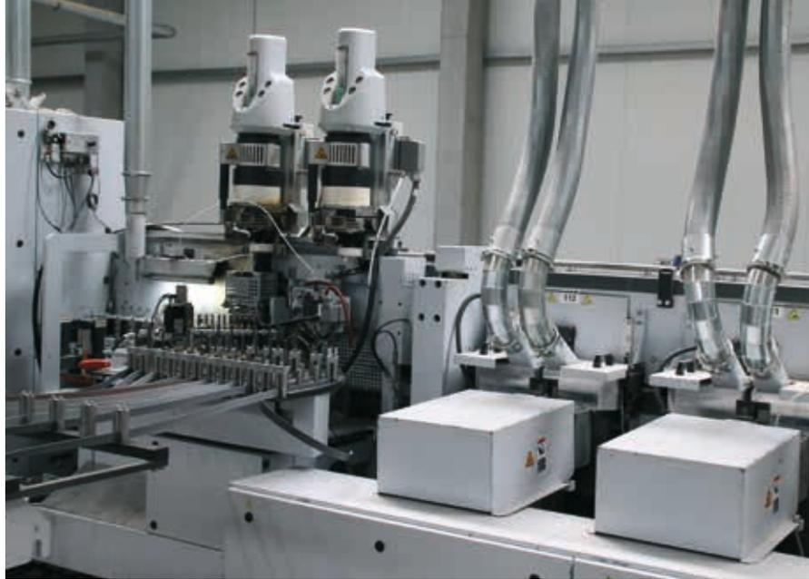
Clearly evident: The four jointing stations on the machine before the edge is then glued to the workpiece.
